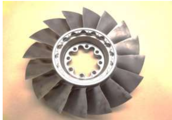
1st stage compressor rotor found with light FOD.
