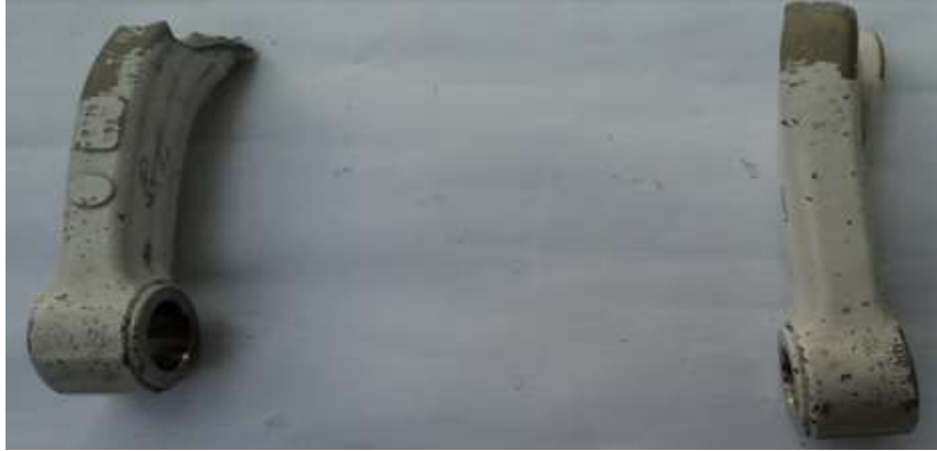
Figure shows nose wheel fork (right and left) parts
