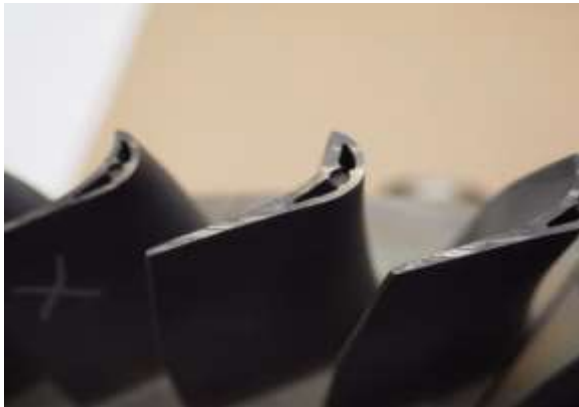
Rubbing observed at the CT blades tip. The inner and outer liner exhibited normal wear.
