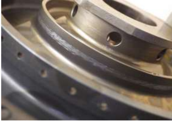
Rubbing at the 1st and 2nd stage PT blades and discs.
