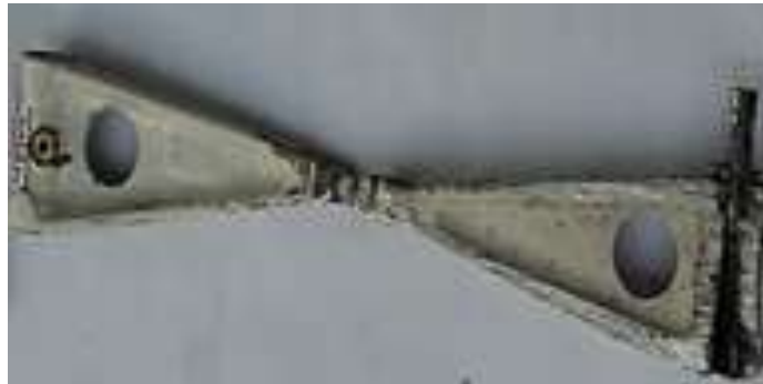
Figure shows lower and upper part of torque link
