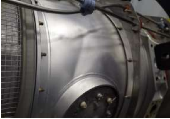
Buckling found at the GG case.
