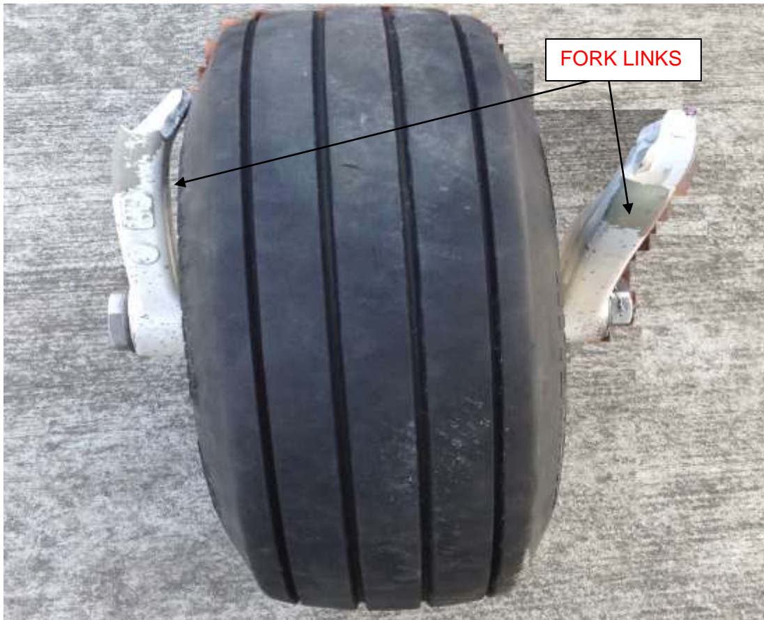
BOTH THE FORK LINKS BROKE DUE IMPACT
