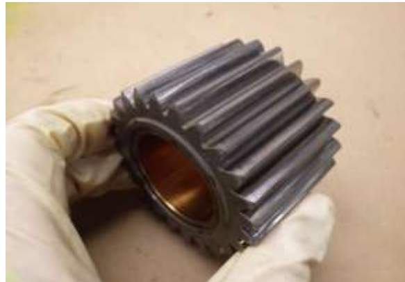
Light wear was observed at the 2nd stage planet gears teeth
