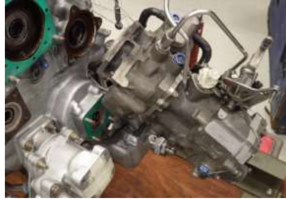
The AGB fuel pump pad was found with broken studs. Engine teared down.
