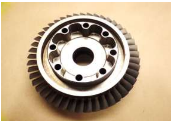
4th stage compressor rotor was found in normal condition (previous cut-back observed) The compressor stator were found with normal wear.
