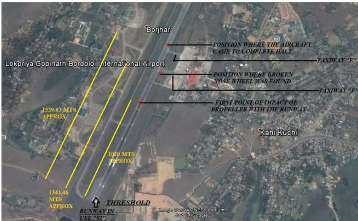
Figure: Location of aircraft and parts on the runway after landing.
