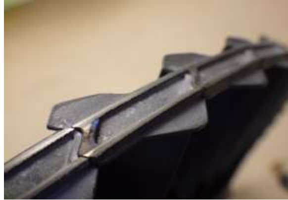
Rubbing at the 1st and 2nd stage PT blades and vanes
