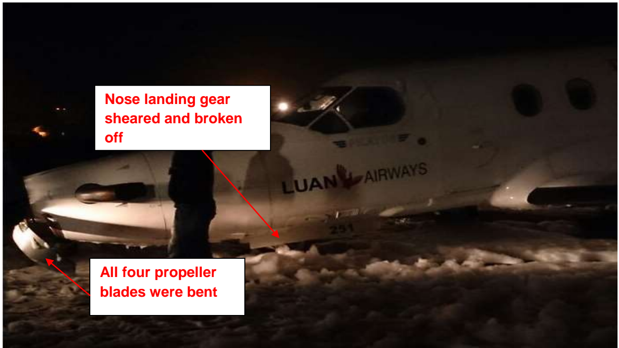
Final resting position of the aircraft on the runway with nose landing gear broken off
