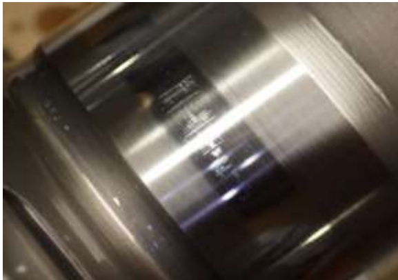
Scores were observed on the 2nd stage carrier at #5 bearing journal.
