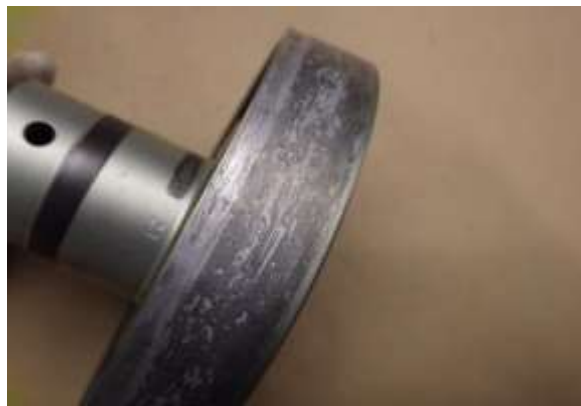
Light rubbing at the rear compressor stub shaft
